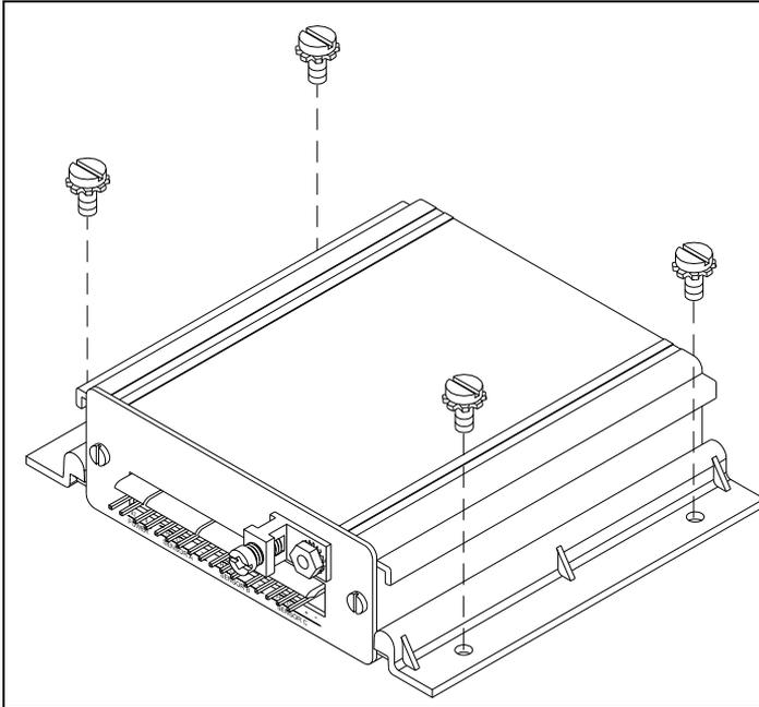
1. Locate the flat surface where the control unit will be mounted. Allow enough clearance at the rear of the unit for mating portion of the rear connectors. Keep in mind that the flexible-core sensor's wire is 2 meters long (6 feet).
