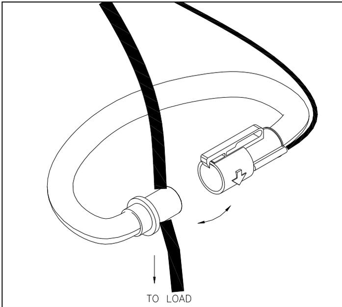
9. Install the flexible-core sensor(s) around the conductor(s), paying close attention to pointing the arrow on the sensor towards the load.
